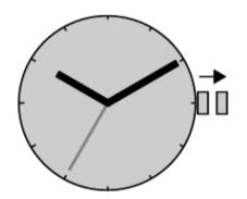
To set your watch's time, simply pull the crown out to the furthest position from the watch base. The second hand stops to help you accurately set the time.
