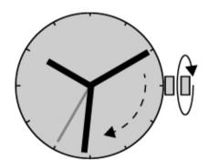
Gently turn the crown clockwise (or away from you) until you set the correct time, with the minute hand 1 minute ahead of the correct time.
