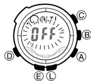
1. In the Altimeter Mode, hold down (E) for about two seconds until either **OFF** or the current reference altitude value starts to flash. This is the setting screen.
